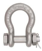
Bolt Type Anchor shackles with thin head bolt – nut with cotter pin. Meets the performance requirements of Federal Specification RR-C-271D Type IVA, Grade A, Class 3, except for those provisions required of the contractor. For additional information, see page 450.
